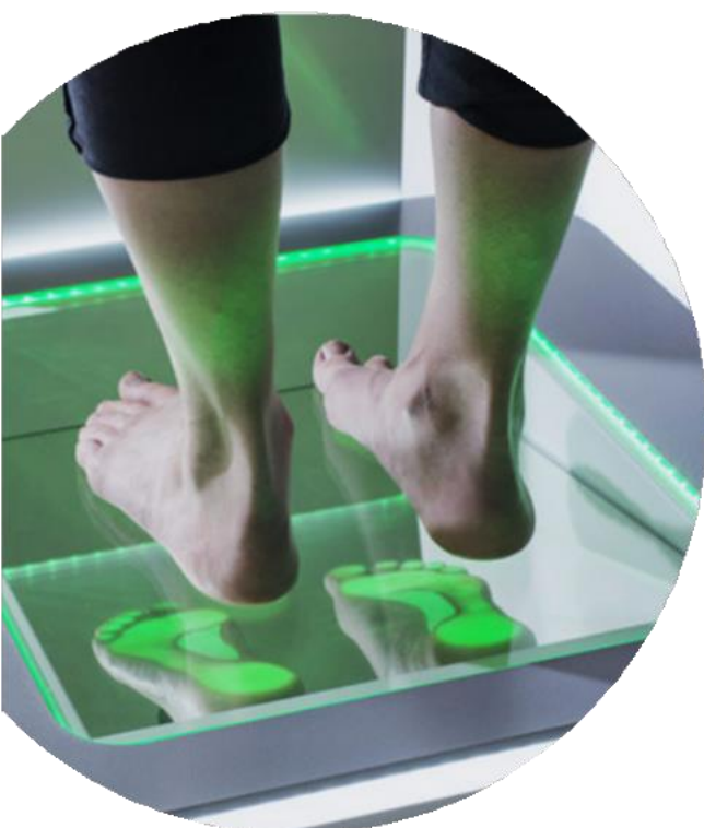
Digital foot scanning process for the production of the adapted shoes.
